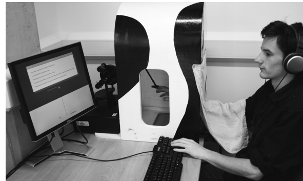
Figure 1. The PHANToM Premium 1.5 and other apparatus as configured for the experiment. Shown on the computer screen are the instructions and a simple visualization of the virtual surface and haptic interaction point presented during the pre-experiment tutorial. No graphical information was shown during the experiment.
