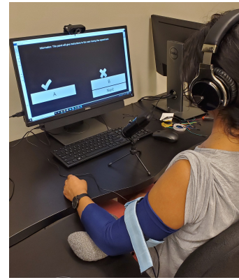
Fig. 2. Participant wearing the tactor band on top of the left biceps. The computer screen shows the interface for pairwise discrimination. Button “A” is associated with the broadband, single-tactor stimulus and button “B” with the narrowband, two-tactor stimulus.
