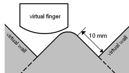
Figure 6. Illustration of the additional walls added to the virtual edges used in the follow-up experiment. The dashed lines show where the two side surfaces used to be, and the gray areas indicate the inside of the virtual object.
