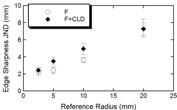
Figure 5. Means and standard errors of edge sharpness discrimination thresholds for all fourteen participants.
