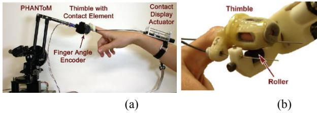
Figure 1. (a) Contact location display system. (b) Side view of the roller in the contact location display. (From Fig.2b in [20], and Fig. 4 in [27], respectively.)
