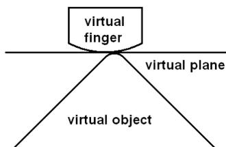
Figure 7. Illustration of virtual objects used in the CLD alone condition. The virtual plane was used in rendering force. The virtual object was used in calculating contact locations.
