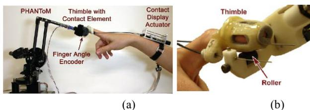
Figure 1. (a) Contact location display system. (b) Side view of the roller in the contact location display. (From Fig.2b in [20], and Fig. 4 in [27], respectively.)
