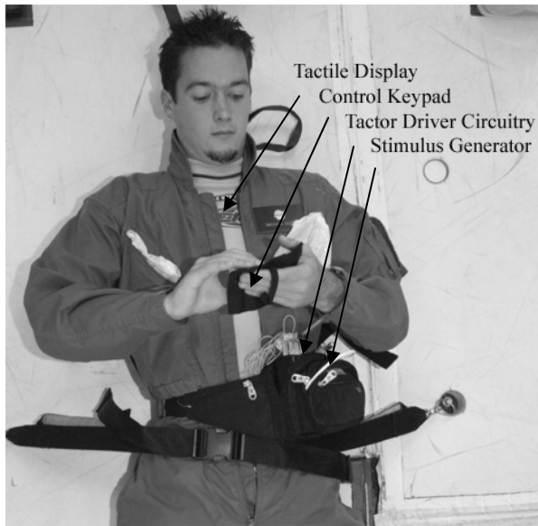
Figure 1. Experimental apparatus. Shown here is one subject conducting the experiment while being strapped to the floor of the KC-135A.
