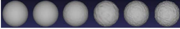
Fig. 3. The six spherical surfaces with increasing roughness used in the present study. The estimated roughness values were 0.000027, 0.000209, 0.001704, 0.003139, 0.010937, and 0.025304, respectively, from left to right. The six spherical surfaces contained the same number of vertices (3752) and faces (7500).
