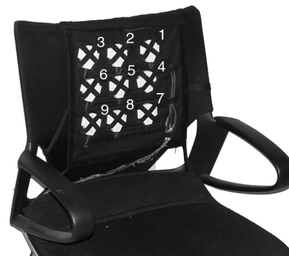
Figure 2. The haptic cueing system. Shown here is a 3-by-3 tactor array draped over the back of a chair.
