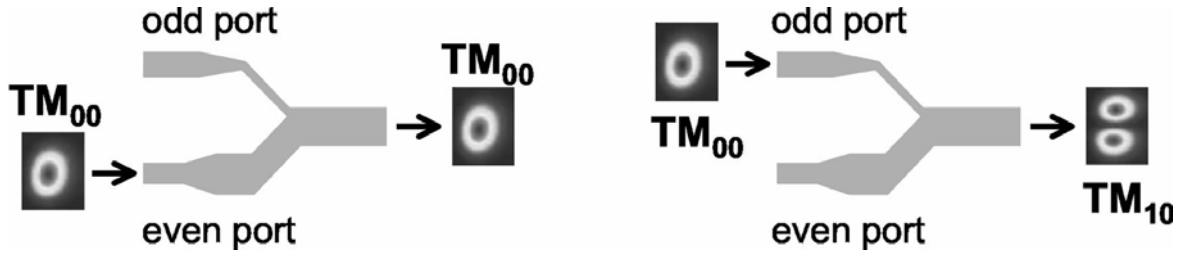
Fig. 5.2. Schematic diagram of mode conversion by asymmetric Y junction [60].
