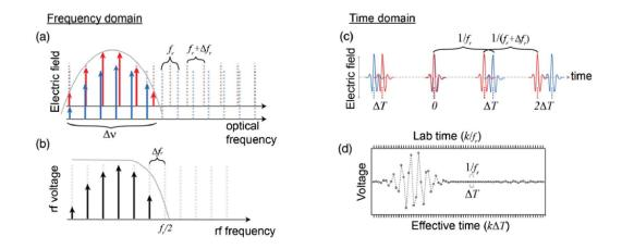
Fig. 1.6.: (a) Optical frequency domain picture of dual comb spectroscopy DCS. (b) RF domain picture of DCS. (c) Time domain visualization of the reference and signal pulses walking through each other. (d) Oscilloscope picture of DCS [60].
