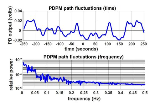
Fig. 4.12.: Measured path length fluctuations through the PDPM when the interferometer is not stabilized. The top plot shows the photodetector (PD) voltage as a function of time. The data was recorded over 500 seconds and sampled every 0.5 ms. The bottom plot shows the spectrum of the path length fluctuations, the spectrum shows that the fluctuations are in the order seconds.
