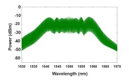
(a) An example spectrum out of a length of highly nonlinear fiber (HNLF), depicting the spectral ripple associated with residual third order phase.
