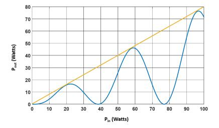
Fig. 2.4.: Plot of NOLM transmission; note the oscillatory behavior.
