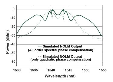
Fig. 2.10.: Simulated spectral results of three PMs and one IM. The two different spectra correspond to either compensation of all orders of spectral phase (solid) or only quadratic spectral phase compensation (dotted).
