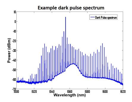
Fig. 5.1.: Example of dark pulse spectrum generated from a normal dispersion microresonator.
