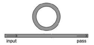
Fig. 1.4.: A cartoon depicting a microring resonator with a bus waveguide [43].
