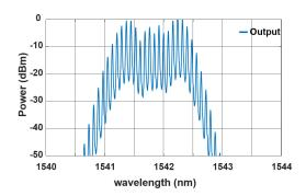
(a) Output spectrum of EO comb generator comprised of one IM and one PM.
