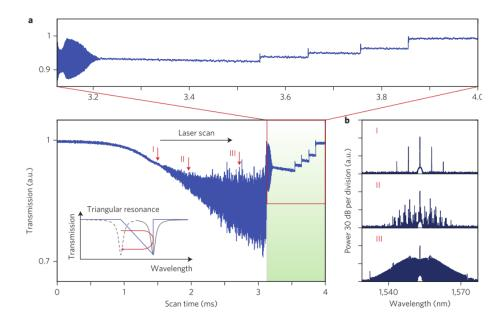
Fig. 3.1.: The signature of soliton generation. The transitions from a noisy chaotic state to N solitons. Further red detuning eventually leads to the single soliton regime [106].
