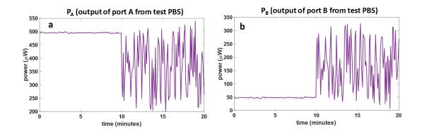
Fig. 4.19.: 20 minute measurement of the polarization stability of the classical light in the forward propagation direction (purple arrow). a - port A of the test PBS. b port B of the test PBS.
