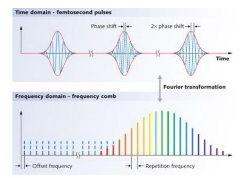
Fig. 1.2.: Cartoon depicting what an OFC looks like in the time domain (top), and in the frequency domain (bottom) [10]. The top figure also depicts the CEO arising from the shift between fast oscillating electric field and pulse envelope.
