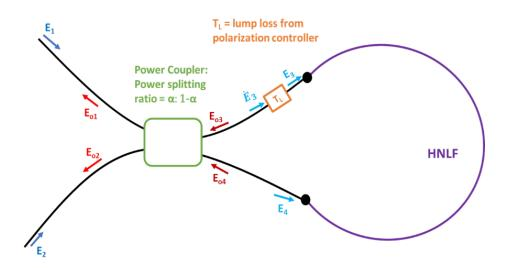
Fig. 2.3.: Cartoon depicting NOLM comprised of a 2x2 power coupler and a length of HNLF. The NOLM is a Sagnac interferometer.
