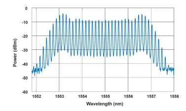
Fig. 3.7.: Spectrum of electro-optic frequency comb generated from two phase modulators and one intensity modulator.
