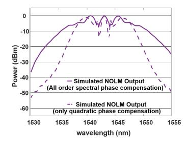
Fig. 2.9.: Simulated spectral results of two PMs and one IM. The two different spectra correspond to either compensation of all orders of spectral phase (solid) or only quadratic spectral phase compensation (dotted).
