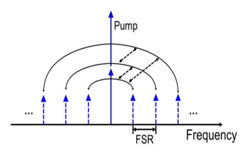
Fig. 1.7.: The general depiction of a biphoton frequency comb (BFC) [90]. A BFC is a coherent superposition of N-energy matched frequency bins.
