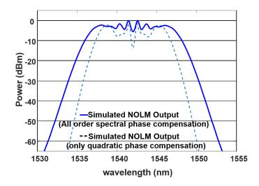
Fig. 2.8.: Simulated spectral results of one PM and one IM. The solid spectrum corresponds to compensating for all orders of spectral phase. And the dotted spectrum corresponds to compensating for only quadratic spectral phase.
