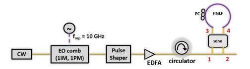
Fig. 2.5.: Experimental setup for removing residual third order wings via the NOLM.
