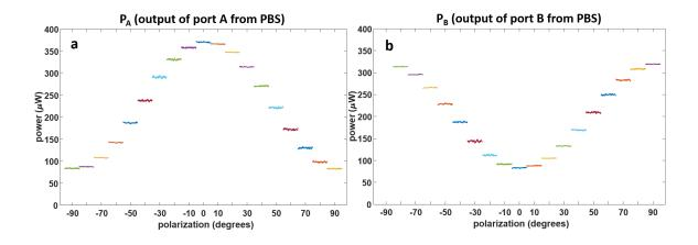
Fig. 4.16.: Polarization stability of the classical light through the test interferometer as its polarization is swept from  $-90^{\circ}$  to  $+90^{\circ}$  in  $10^{\circ}$  increments. Power is recorded out of each port of the test PBS for 10 minutes at each polarization setting. a – port A of the test PBS. b – port B of the test PBS.
