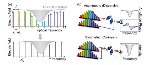
Fig. 1.5.: (a) Cartoon depicting the basic concept of dual comb spectroscopy (DCS). The goal of DCS is to map the optical information to the RF domain. (b) The two types of DCS, asymmetric and symmetric [60].
