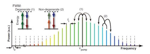
Fig. 1.3.: Depiction of the two types of four wave mixing taking place inside a microresonator, degenerate and nondegenerate four wave mixing [38].
