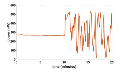
Fig. 4.14.: 20 minute measurement of the output power of the stabilization laser (backwards path - orange arrows). This shows the interferometer being stabilized for the first 10 minutes and not being stabilized for last 10 minutes. For the data with stabilization on, the standard deviation of the fluctuations is 2.57  $\mu$ W, and for the stabilization off data the standard deviation is 150.36  $\mu$ W.
