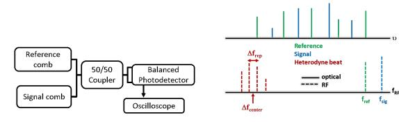
(a) Generalized setup for dual comb EFXC measurement.
