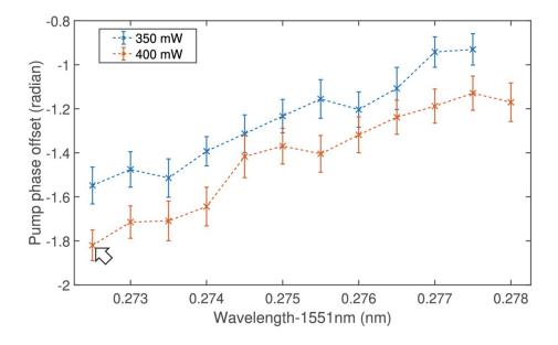
Fig. 3.13.: Results of pump line phase offset study with increasing pump wavelength. The data point indicated by the arrow corresponds to the data presented in figure 3.12c.
