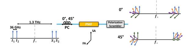
Fig. 4.9.: The effect of the polarization scrambler on the polarization state of the frequency-bin pairs when the launch condition is changed from  $0^{\circ}$  to  $45^{\circ}$ . PC – polarization controller and PMF – polarization maintaining fiber. The polarization scrambler effectively rotates the global polarization of the BFC.
