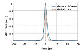
(b) Comparison of measured and expected AC trace of compressed pulse out of the EO comb. All orders of spectral phase were compensated for in the pulse compression.
