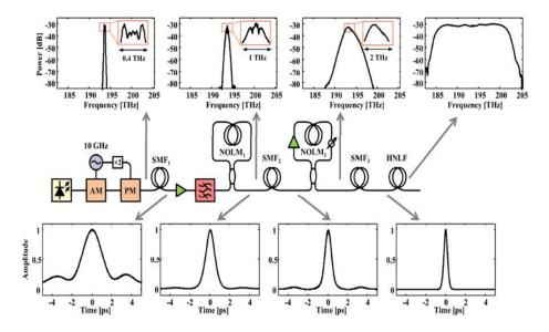
Fig. 2.2.: Experimental setup for spectral broadening employing one NOLM stage and one NALM stage. [93].
