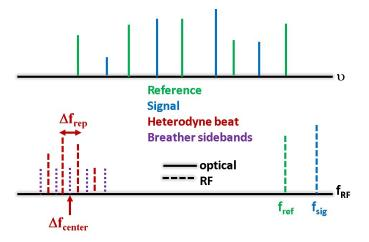
Fig. 5.2.: We expect to visualize the breathing dynamics of the dark breather by observing (purple) sidebands on the retrieved RF comb from the Dual Comb EFXC measurement.
