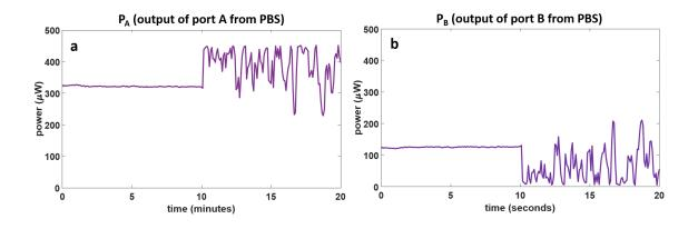
Fig. 4.15.: 20 minute measurement of optical power of classical light (forward propagation - purple arrows). This shows the interferometer being stabilized for the first 10 minutes and not being stabilized for last 10 minutes. The polarization setting on the DPC is set to a polarization ensuring light through both arms of the PDPM and causes this power imbalance between output ports of the test PBS. a - port A of the test PBS, b - port B of the test PBS.
