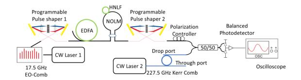
Fig. 3.11.: The experimental setup for performing dual comb interferometry for characterization of single-soliton Kerr-comb [103].
