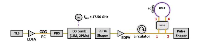
Fig. 3.6.: Experimental setup for spectrally broadening electro-optic frequency comb for use as reference comb in the dual comb interferometry measurements.
