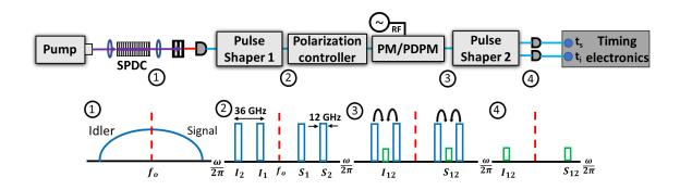
Fig. 4.3.: Experimental setup for measuring frequency-bin entanglement in a BFC. Note that either a standalone phase modulator (PM) or polarization diversity phase modulator (PDPM) is used to mix frequencies in this arrangement.
