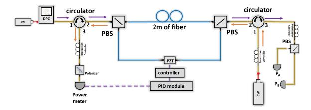
Fig. 4.13.: Setup to achieve and show active stabilization of classical light in an interferometer. DPC - deterministic polarization controller, PBS - polarization beam splitter, CW - continuous wave laser, PZT - piezo electric transducer (fiber phase shifter), PID - proportional integration derivative.  $\lambda_{CW_1} = 1555$  nm and  $\lambda_{CW_2} = 1545$  nm.
