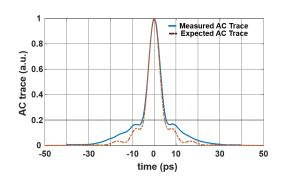
(b) Comparison of measured and expected AC trace of the compression out of EO comb generator. Only quadratic spectral phase was compensated for.
