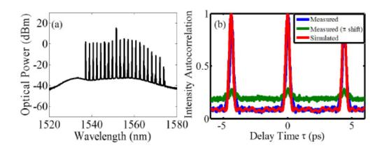
Fig. 3.3.: (a) Optical spectra after EDFA and pulse shaper for pump wavelength of 1551.27nm (b) Autocorrelation data (blue) and simulation (red) based on measured spectrum assuming flat phase. Autocorrelation data with  $\pi$  phase shift applied to the pump (green).
