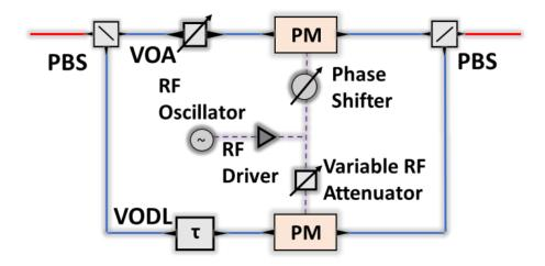
Fig. 4.1.: Schematic of the polarization diversity phase modulator (PDPM) – singlemode and polarization-maintaining fiber are depicted in red and blue, respectively. PBS - polarization beam splitter, VOA - variable optical attenuator, VODL - variable optical delay line, PM - phase modulator.
