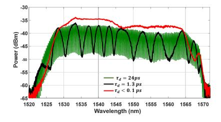
Fig. 4.2.: Progression of spectral ripple removal, signifying balancing the lengths of the arms of the PDPM.
