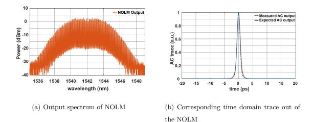
Fig. 2.7.: (a) Spectrum out of the NOLM. (b) Corresponding time domain trace out of the NOLM; notice the removal of the third order dispersion wings.
