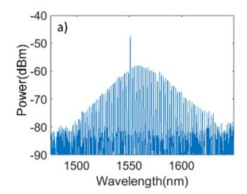
Fig. 3.5.: Single soliton generated in SiN microring resonator depicted in figure 3.2. This spectrum is taken from the drop port. Note the slight offset of the pump line arising from Raman interactions. The free spectral range (FSR) is 227.5 GHz.
