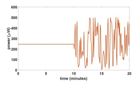
Fig. 4.18.: 20 minute measurement of stabilization laser output. The first ten minutes are with stabilization on (and RF delay balanced), and the last ten minutes are with stabilization off. For the data with stabilization on, the standard deviation of the fluctuations is 0.032  $\mu$ W, and for the stabilization off data the standard deviation is 152.36  $\mu$ W.
