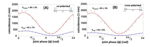
Fig. 4.10.: Interference traces and visibilities from measurements of frequency-bin entanglement in a BFC. The performance of a standalone PM (blue) was compared with that of the PDPM (red). The experiments were carried out for both co– (A) and cross–polarized (B) signal idler pairs.
