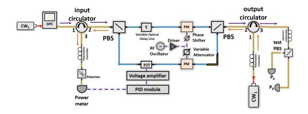
Fig. 4.17.: Experimental setup for active stabilization of the PDPM. The RF components necessary to balancing the PDPM electrically are now incorporated. This setup is used to demonstrate that the polarization transformation observed in figure 4.21 is due to the RF delay mismatch between the PMs.
