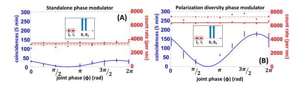
Fig. 4.7.: Frequency-bin entanglement measurements on orthogonally polarized signal-idler pairs using (A) a standalone PM and (B) the PDPM. Dashed and solid red lines correspond to the signal and idler count rates, respectively. The insets show the relative orientation between the polarization of signal and idler bins.
