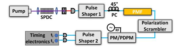
Fig. 4.8.: Experimental setup for state preparation and measurement of frequencybin entanglement. PC – polarization controller and PMF – polarization maintaining fiber.
