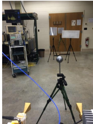
Fig. 3.6 Photograph of the experimental setup of the ultra-high resolution W-band ranging experiments
