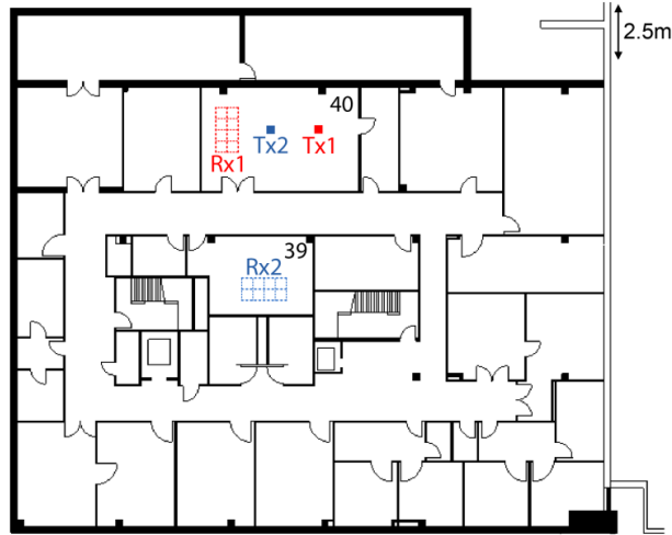
Fig 3.1: Environment layout. Tx1 and Rx1 show respectively the positions of the transmitter and the receiver grid for the LOS measurements. Tx2 and Rx2 are the corresponding locations for the NLOS experiments.
