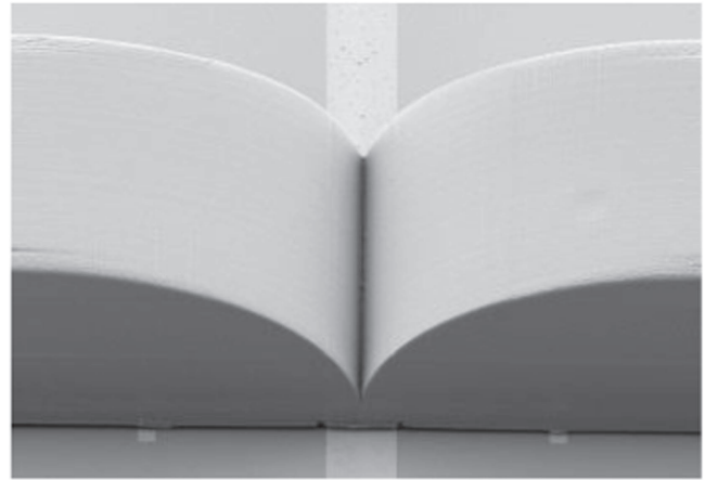
Figure 27. Electron micrograph of a fabricated cloak for a metal contact ( 20\ \mu\text{m} width) on a silicon surface. The structure has been designed by mapping a 1D coordinate transformation onto a dielectric (polymer) free-form surface, which refracts the incident light such that it avoids the metal contact. Reproduced with permission from [148].
