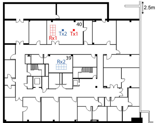
Fig. 2. Environment layout. Tx1 and Rx1 show respectively the positions of the transmitter and the receiver grid for the LOS measurements. Tx2 and Rx2 are the corresponding locations for the NLOS experiments.
