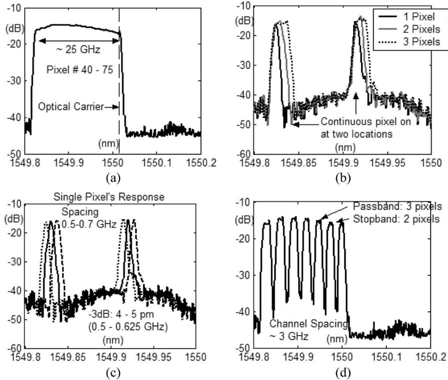
Fig. 3. Characterizations of programmable optical filters based on a virtually imaged phased-array. (a) Transmission response with pixel #40–#75 turned on, (b) single pixel response versus double or triple continuous adjacent pixels' response, (c) single pixel response at three continuous adjacent pixels, respectively, and (d) an example of optical comb filtering.
