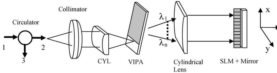
Fig. 2. Experimental setup of our programmable coherent optical filter based on a virtually imaged phased-array: cylindrical lenses (CYL) and spatial light modulator (SLM).
