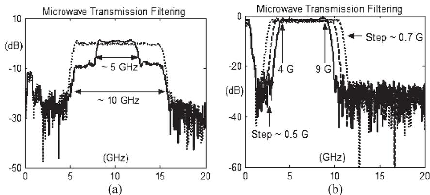
Fig. 5. Engineerable microwave filtering. (a) Microwave bandpass filtering with stepped response and (b) microwave bandpass filtering compatible to UWB spectral range 3.1–10.6 GHz.
