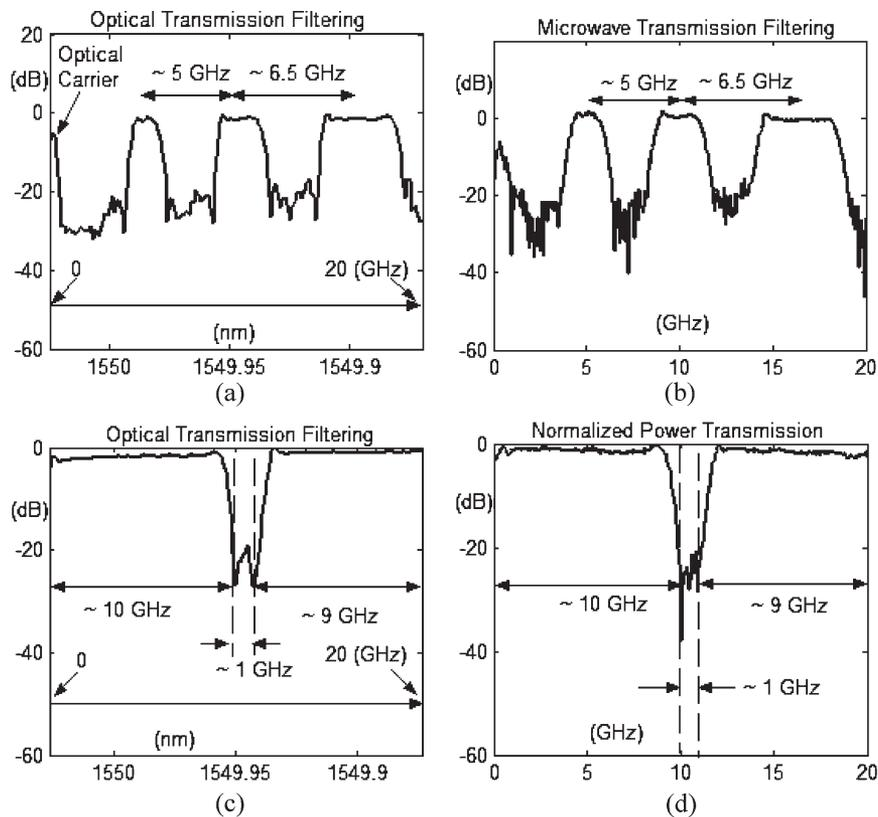
Fig. 4. Correspondence between optical filtering and microwave filtering. (a) Optical multipassband filtering, (b) corresponding microwave multipassband filtering, (c) optical notched filtering, and (d) corresponding microwave notched filtering.
