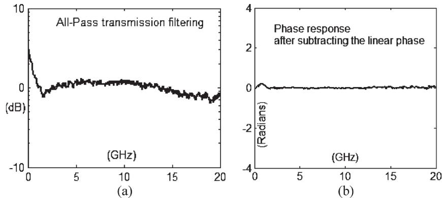
Fig. 6. Phase response of programmed microwave filters. (a) All-pass power transmission without amplitude modulation and (b) corresponding phase response for all-pass filtering.
