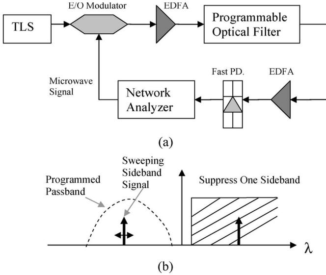
Fig. 1. (a) Experimental setup for photonic processing of microwave signals. Tunable laser source (TLS) and erbium doped fiber amplifier (EDFA). (b) Optical spectral sketch to illustrate the general principle of photonic processing.
