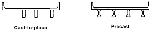
Fig. 2.5.3.2-Cross sections of stringer bridges
