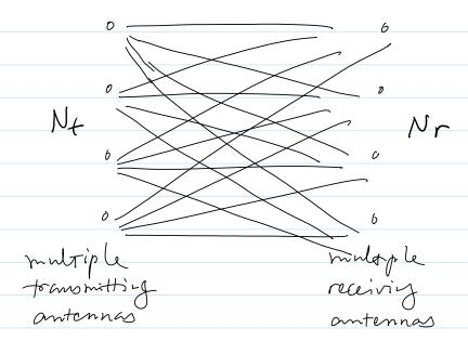
If the channel matrix is "right", the data rate can grow as min (Nt, Nr)
