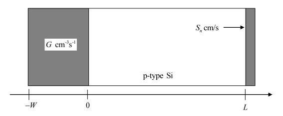
Assume that the electron-hole generation rate is G for  $x \le 0$  and that the contact at x = L is specified by a minority carrier surface recombination velocity  $S_n$ .
