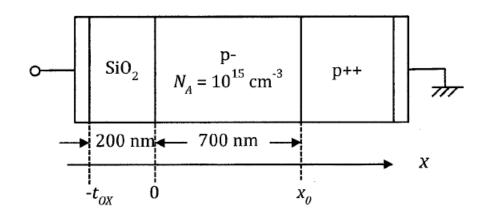
Compute the surface potential required to produce a depletion width of 500 nm.
