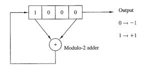
Figure P2.65 Linear feedback shift register.
