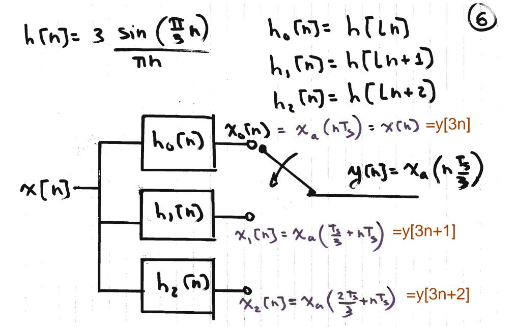
In this set of notes,  $x_0$  [n],  $x_1$  [n] and  $x_2$  [n] represent the fractional time-shift filter outputs in the case of upsampling ONE signal.
