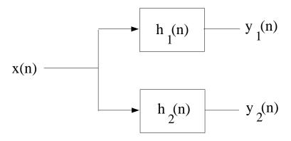
Consider the system above where the causal signal x(n) is simultaneously input to two different causal FIR filters of length M = 2 with respective impulses responses  $h_1(n)$  and  $h_2(n)$ . That is, both  $h_1(n)$  and  $h_2(n)$  are only nonzero for n = 0 and n = 1. We don't know anything about the input signal x(n) except that it is causal. Yet, it is possible to determine  $h_1(n)$  and  $h_2(n)$  (to within a scalar multiple) given the respective outputs  $y_1(n)$  and  $y_2(n)$ .
