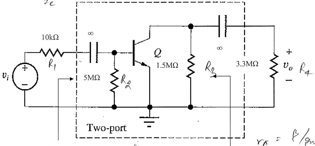
$$g_m = \frac{I_C}{V_T} = \frac{2\mu A}{25m} = \frac{200 \times 10^{-5}}{25} = 8 \times 10^{-5} \text{ S}$$
