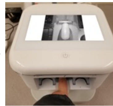
Take picture of the bounding box with fingernail within as PGM, send to Nail Segmentation module
