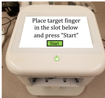
Prompt to get customer to insert finger into the slot for nail capture
