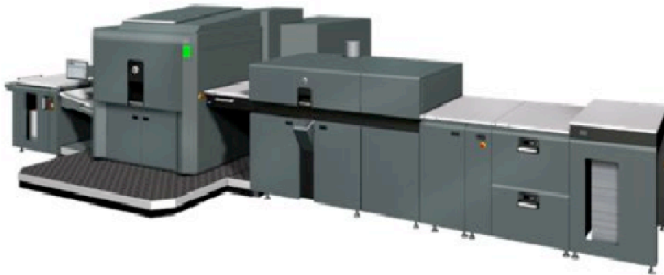
Fig. 2(b) HP Indigo Press 30000, which can print 4600 3-color sheets/hr.
