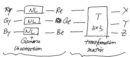
JPA comment: I would describe **characterization** as the process of determining both NL\_i, i = R, G, B and T for the scanner; and calibration as the process of implementing the model shown here to obtain CIE XYZ for a specific scanner RGB
