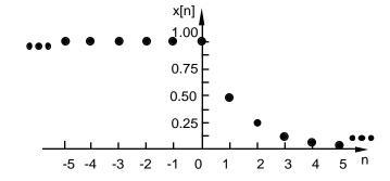
b. A causal, linear, time-invariant discrete-time system has impulse response  $h[n] = 2^{-n}u[n]$ . The response to an unknown input x[n] is  $y[n] = (-1)^nu[n]$ . Find the input x[n].
