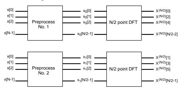
Here the entire N point data sequence x[n] is preprocessed in two different ways to yield two different N/2 point data sequences  $x_0[n]$  and  $x_1[n]$ . Taking the N/2 point DFT of  $x_0[n]$  yields  $X^{(N)}[k]$  for even values of k; and taking the N/2 point DFT of  $x_1[n]$  yields  $X^{(N)}[k]$  for odd values of k.
