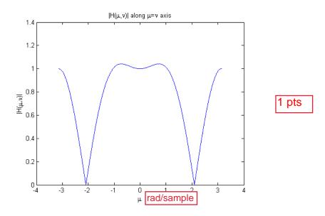
c.  $H(\mu,\nu)$  along  $\mu$  axis is a low-pass filter with a slow roll-off. This filter smoothes the edges in the vertical direction. This can be seen at the bottom portion of the filtered image.
