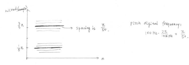
This is a narrowbard spectrogram. The long (too) time window length gives good frequency domain resolution but poor time domain resolution.
