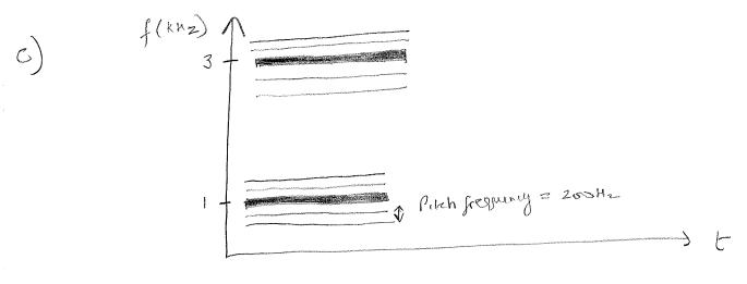
This is a narrow band spectrum breauce we have a larger time window larger which gives good frequency domain resolution but poor time domain resolution
