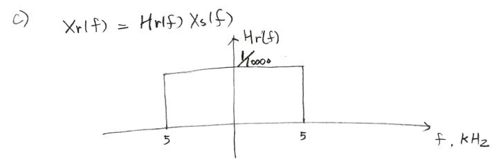
After the low pass filter, only base band survive, and impulses frequence < 5 kHz survives.
