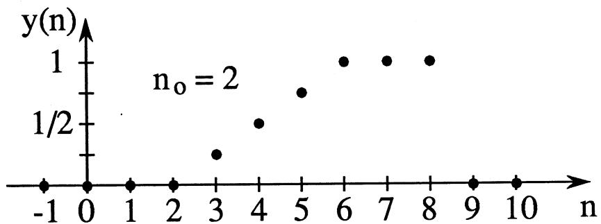
Note that  $n_0$  must be an integer. Non-integer delays can only be defined in the context of a CT signal, and are implemented by interpolation.
