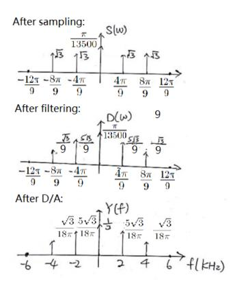
Since the input signal and the low pass filter are the same as part a, the low pass filtered signal for part b is the same as part a.
