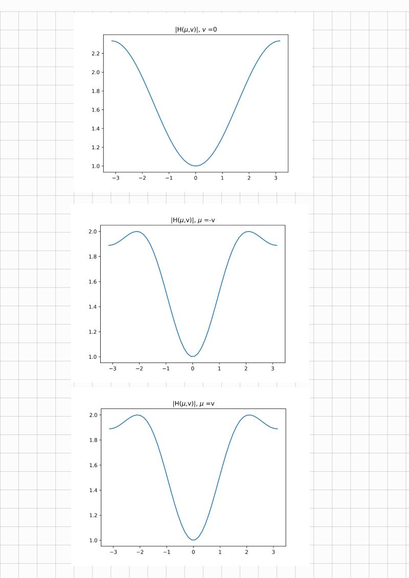
(C) The center region of 1's is preserved, Since this filter is DC preserving The filter is a high pass fifter along both a M 4 V - axoes 4 thus preserves and the edges of i's which can be observed from g tm. 7 7 - s thong the U=V& U=-V the filter accentuete the output first & then dangers it which is visible from the diagonal elements. (d) Yes itid DC preserving because,  $\sum_{m} \sum_{n} h(m,n) = 1.$
