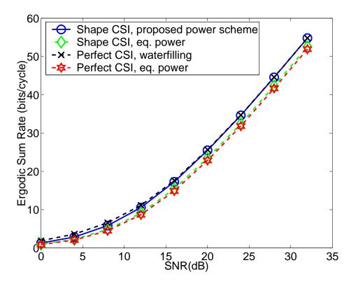
Fig. 3. Ergodic performance of  $R_{\rm sha}^{ci}$ ,  $R_{\rm sha}^{ci-eq}$ ,  $R_{\rm sha}^{ci-eq}$ , and  $R_{\rm sha}^{ci-eq}$  with respect to SNR for N=8 and K=8.
