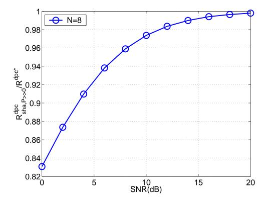
Fig. 1. The ergodic ratio of  $R_{{\rm sha},P>>0}^{dpc}$  to  $R^{dpc*}$  with respect to SNR for N=8 and K=8.
