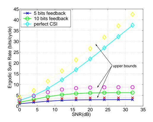
Fig. 5. Ergodic sum rate of limited feedback with ZFDPC (in solid lines) and the upper bound (in dashed lines) for N=4 and K=4.
