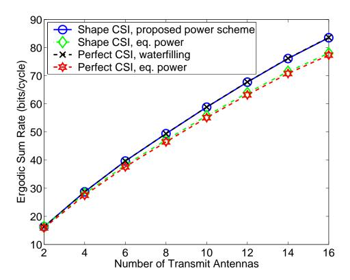
Fig. 4. Ergodic performance of  $R_{\rm sha}^{ci}$ ,  $R_{\rm sha}^{ci-eq}$ ,  $R^{ci*}$ , and  $R^{ci-eq}$  with respect to N for  ${\rm SNR}=30\,{\rm dB}$ .
