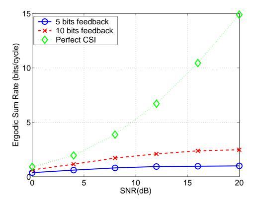
Fig. 6. Ergodic sum rate of limited feedback with channel inversion for N=4 and K=4.
