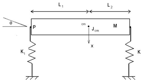
**Determine the modal frequencies, undamped natural frequencies of oscillation, and the modal vectors.**
