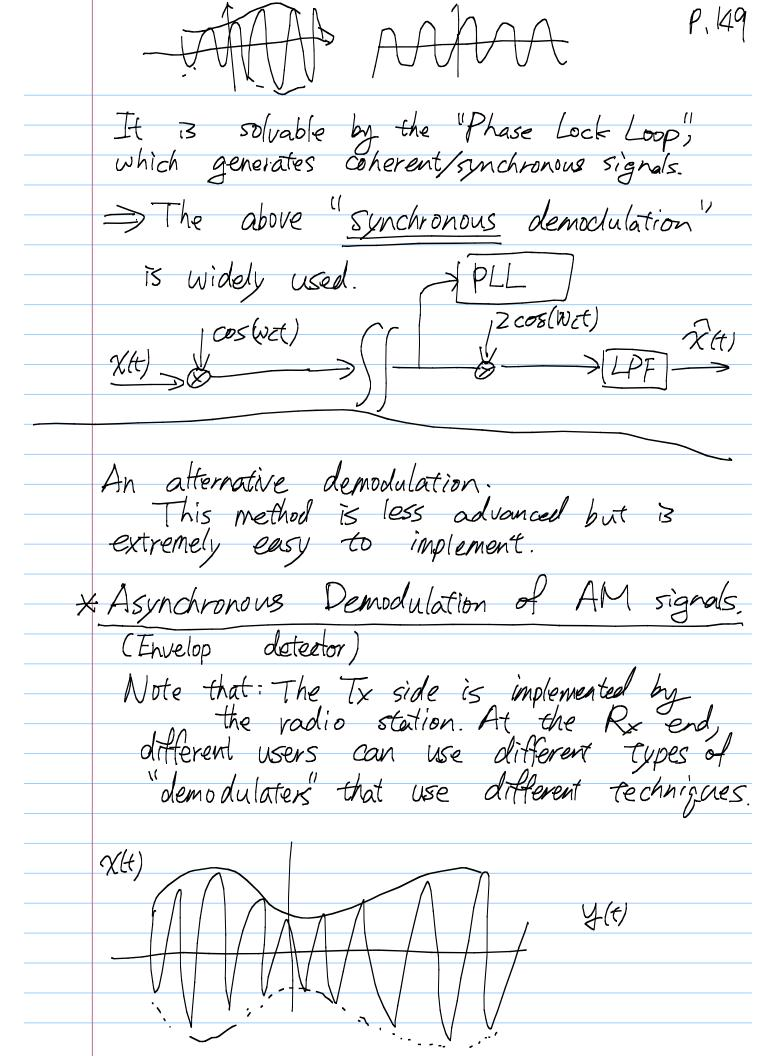
If the carrier signal oscillates much faster than x(t), then x(t) is the "envelope" of the wave form, which can be obtained by "half-wave rectification" (see p. 590-594).
