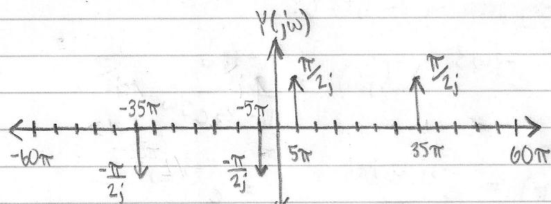
3. 5Hz  $\rightarrow \omega_0 = 2\pi f_0 = 2\pi \cdot 5 = 10\pi \rightarrow \text{cutoff at } 10\pi = \omega$
