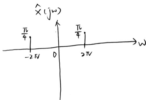
$\hat{x}(t)$  has a lower volume than  $x(t)$ . We can make the low pass filter used for descrambler,  $h_2(t) = 4h(t)$ .
