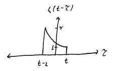
$$y(t) = \int_{t-2}^{t} 2^{\gamma} 2^{t-\gamma} d\gamma = 2^{t} \int_{t-2}^{t} d\gamma = 2^{t+1}$$
