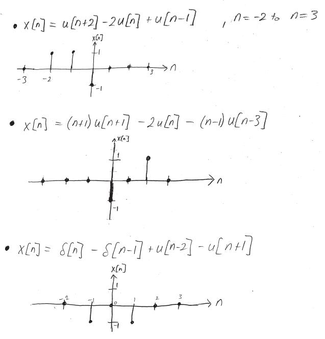
The above signal graph for 8(c) is incorrect. The correct graph is given below.
