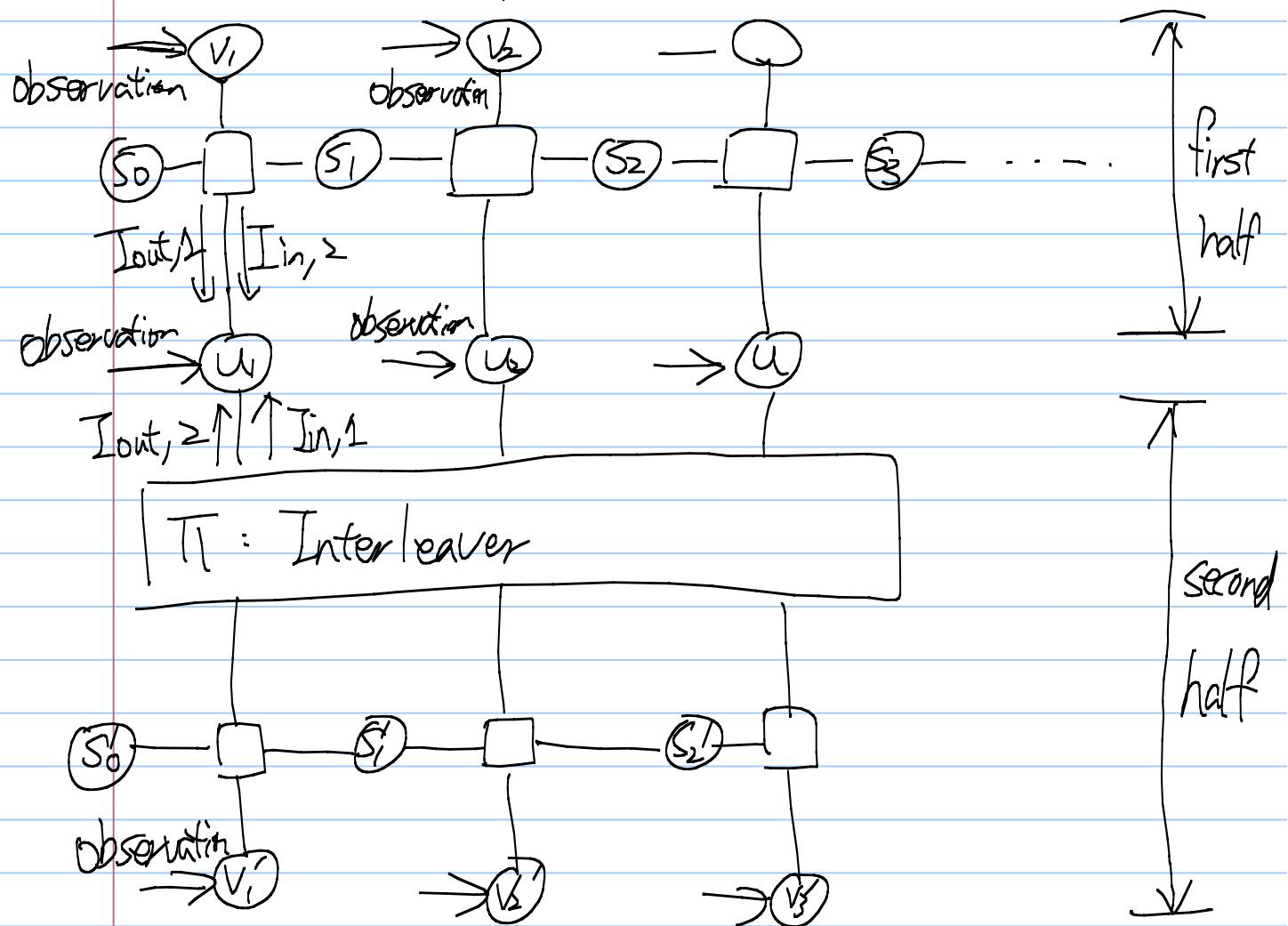
EXIT Chart: <sup>①</sup> Separating the turbo code into two components
