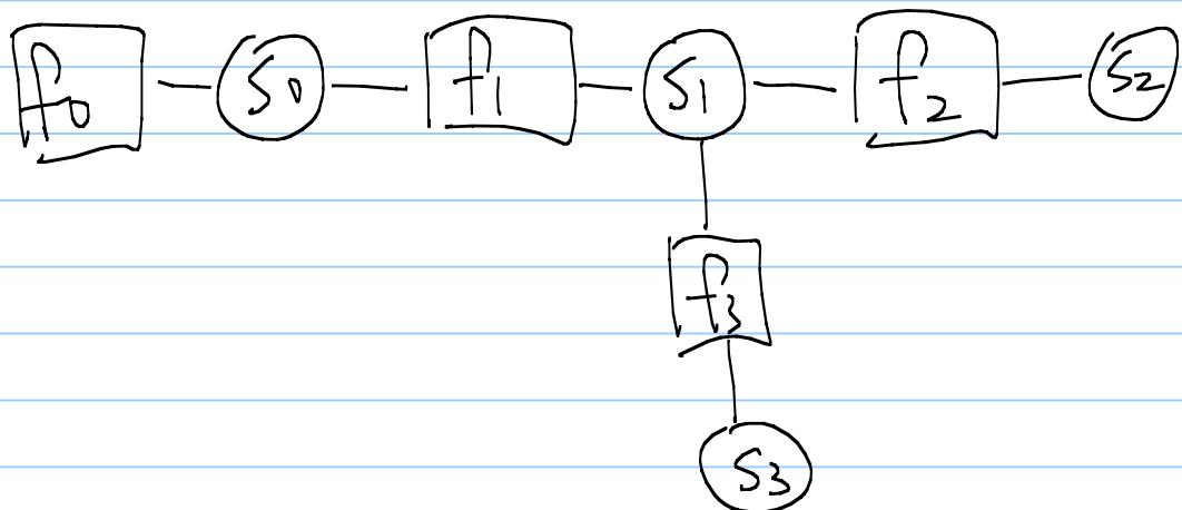
② Initialize the  $f_0 \dots f_3$  functions by the trellis structure & by the observation  $\tilde{y}$
