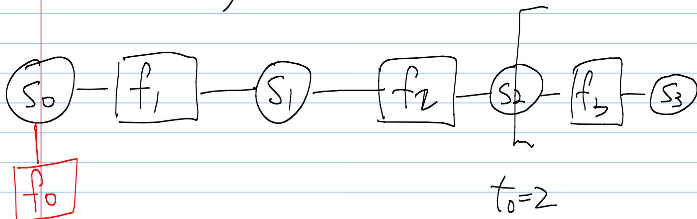
$$t_0=2. \quad b_S[2] \triangleq b_{S_2} = \max_{S_3} f_3(S_2, S_3) b_{S_3}$$
