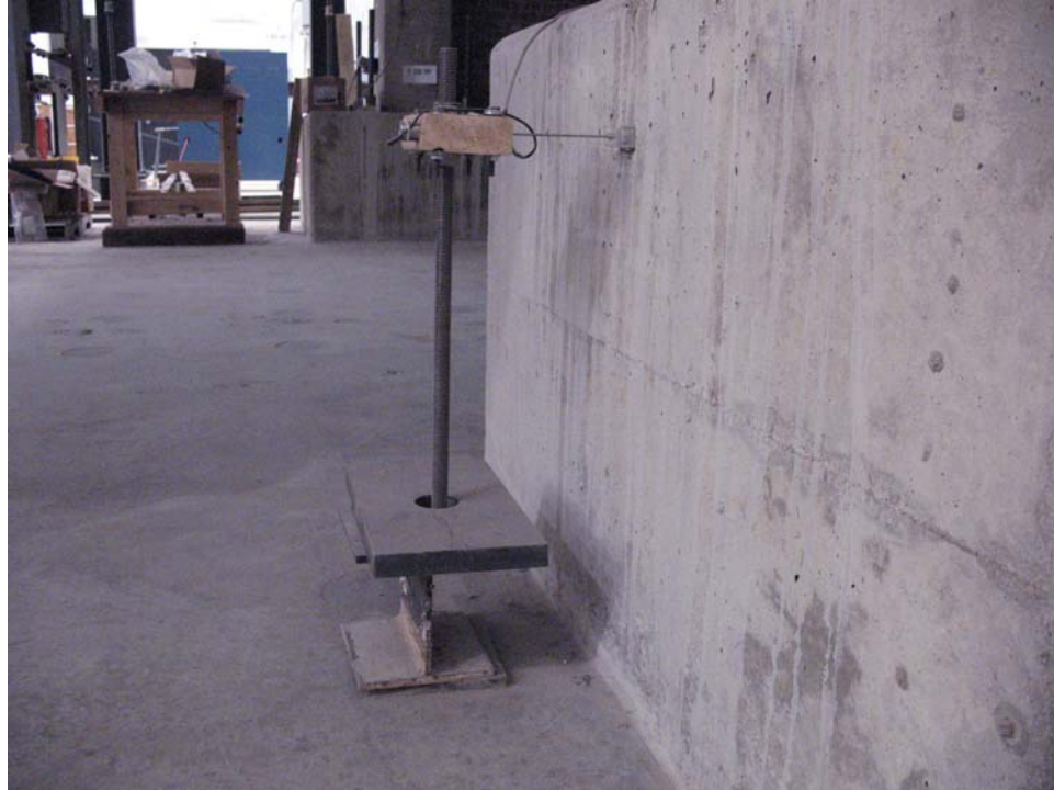
Figure A-31 Footing Movement LVDT
