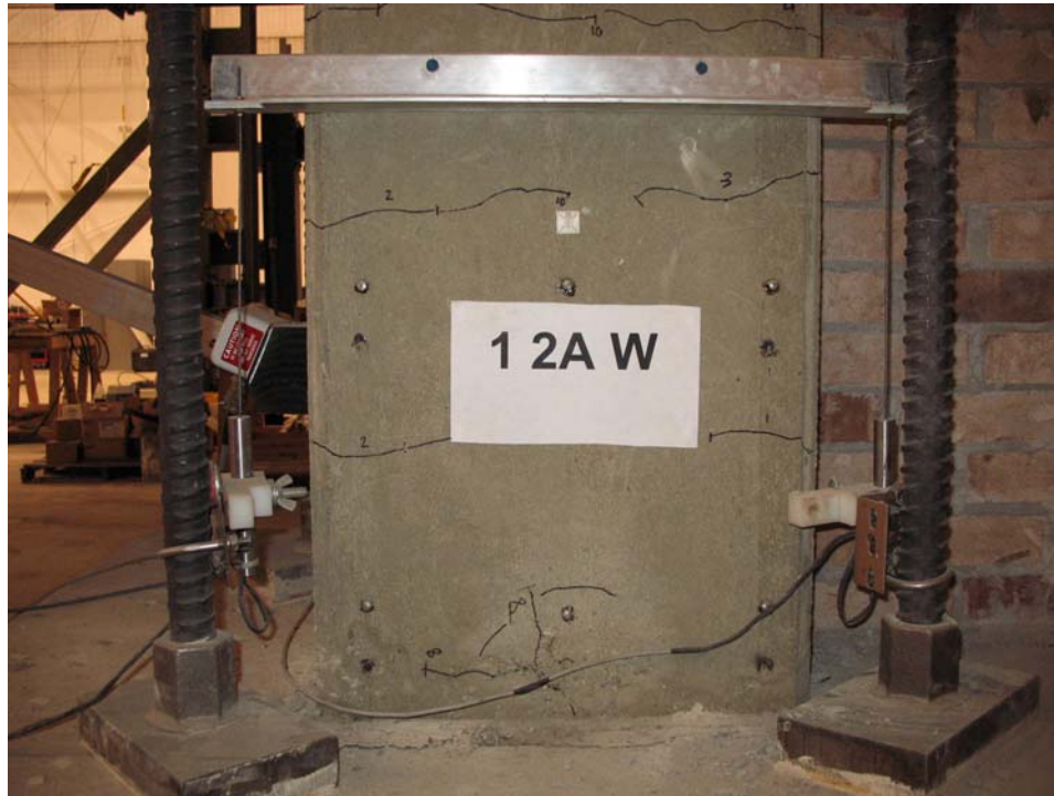
Figure A-30 Column Rotation LVDT
