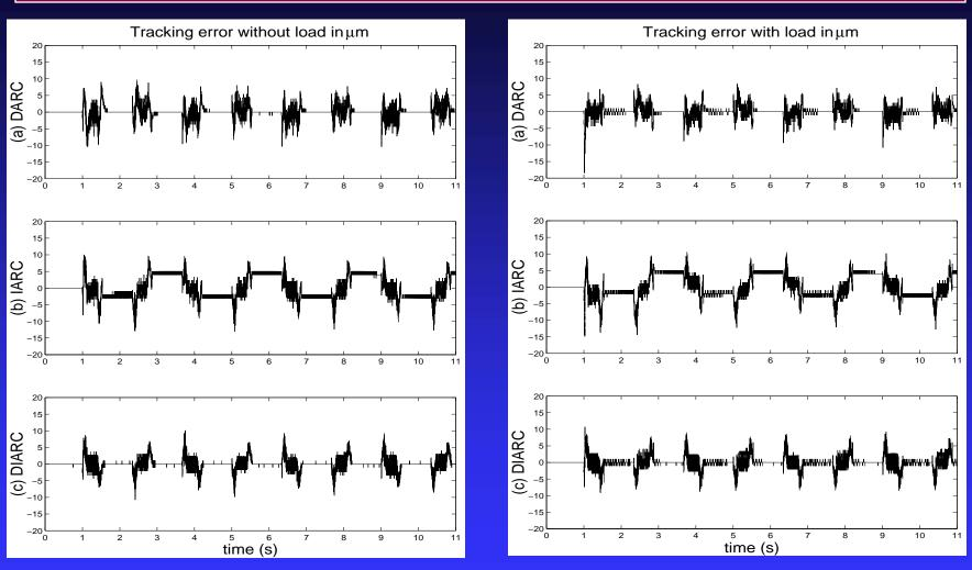
The above results demonstrate the excellent robust tracking performance of the proposed ARC algorithms – Tracking errors are mostly within 10 micrometers with final tracking error around the encoder resolution of 1 micrometer for both loaded and unloaded cases
