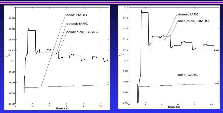
On-line estimates of the Coulomb friction converge to their actual values for both loaded and unloaded cases
