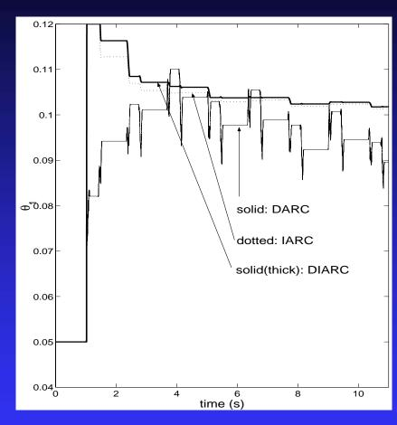
The above plots show the accurate parameter estimation capability of the proposed DIARC and IARC – estimates of the inertia load converge to their actual values for both loaded and unloaded cases
