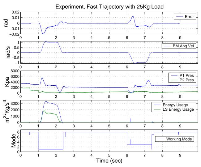
Note that no pump energy is used for boom down motion, and even with the cheap cartridge valves, maximum position tracking error less than 0.02 rad is achieved
