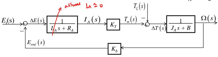
$$\Omega(s) = \frac{\frac{K_{T}}{L_{A}J_{A}}}{s^{2} + \left(\frac{B}{J_{A}} + \frac{R_{A}}{L_{A}}\right)s + \left(\frac{R_{A}B}{L_{A}J_{A}} + \frac{K_{T}K_{b}}{L_{A}J_{A}}\right)} \cdot E_{i}(s) - \frac{\frac{1}{J_{A}}s + \frac{R_{A}}{L_{A}J_{A}}}{s^{2} + \left(\frac{B}{J_{A}} + \frac{R_{A}}{L_{A}}\right)s + \left(\frac{R_{A}B}{L_{A}J_{A}} + \frac{K_{T}K_{b}}{L_{A}J_{A}}\right)} \cdot T_{L}(s)$$
