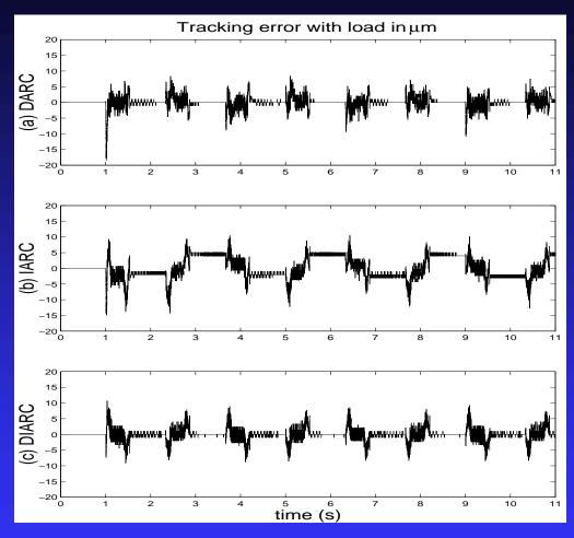
The above results demonstrate the excellent robust tracking performance of the proposed ARC algorithms – Tracking errors are mostly within 10  $\mu$ m with final tracking error around the encoder resolution of 1  $\mu$ m for both loaded and unloaded cases
