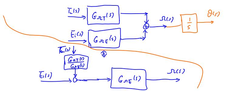
• Substitute the transfer functions' label with the actual formula and simplify
