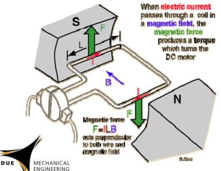
Motors are actuation devices (actuators) generating *torque* as actuation.
