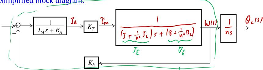
Transfer Function from input voltage  $E_i(s)$  to angular position of the load  $\theta(s)$ :
