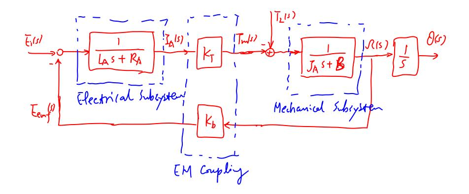
Q: Now that we generated a block diagram of a voltage driven DC Motor, can we derive the transfer function of this motor from its block diagram? (This is the same as asking you to reduce the multi-block diagram to a simpler form just relating inputs  $e_i(t)$  and  $\tau_L$  to the output, either  $\omega$  or  $\theta$ )
