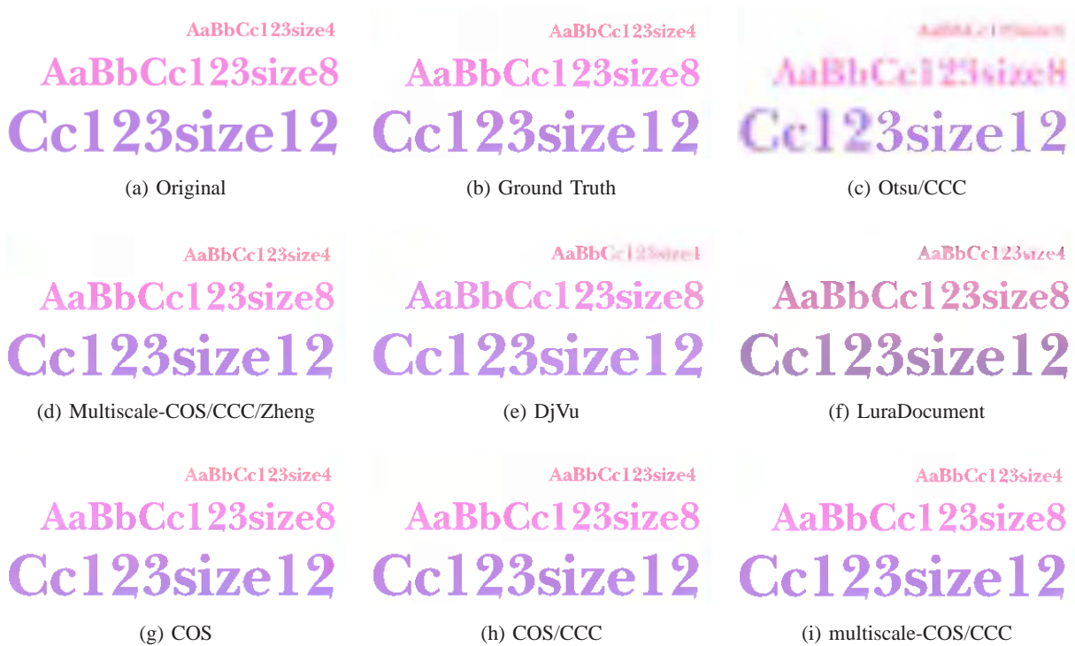
Fig. 13. Decoded MRC image of text regions (400 dpi). (a) Original test image (b) Ground truth (300:1 compression) (c) Otsu/CCC (311:1 compression) (d) Multiscale-COS/CCC/Zheng (295:1) (e) DjVu (281:1) (f) LuraDocument (242:1) (g) COS (244:1) (h) COS/CCC (300:1) (i) Multiscale-COS/CCC (289:1).
