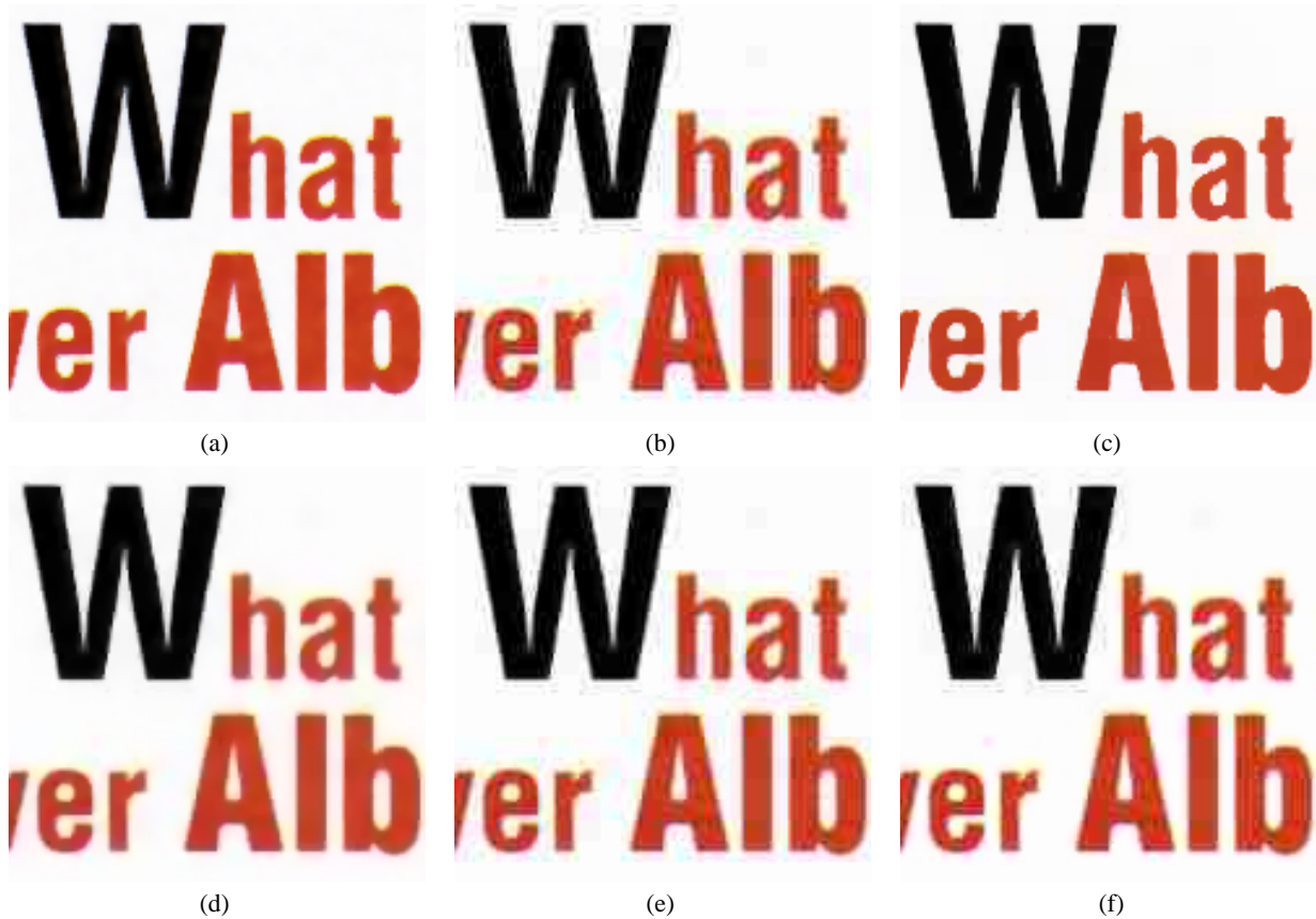
Fig. 15. A text region from Image 3. (a) Original. (b) Conventional JPEG decoding (c) The proposed algorithm. (d) Algorithm I [11]. (e) Algorithm II [34]. (f) Algorithm III [3]. For (f), only the text in red is decoded by the text decoding scheme of Algorithm III. The portion of the document corresponding to the letter “W” is decoded as picture by Algorithm III.
