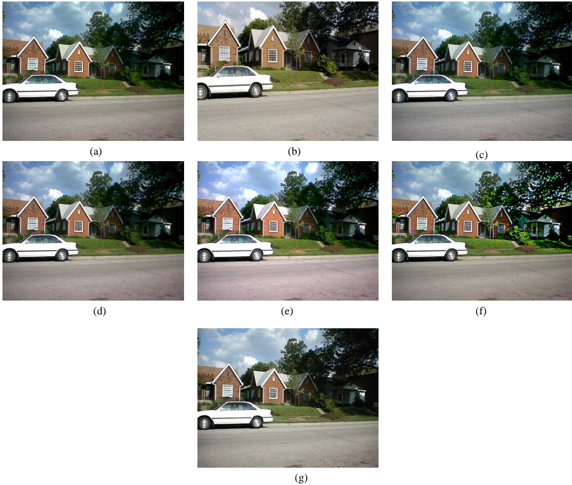
Fig. 13. Image-4, outdoor scene, classified as having no dominant color cast. (a) Camera phone image (Nokia 3650). (b) Reference Image (Nikon D-100). Processed images using (c) “Auto Color” in Adobe PhotoShop ® 7.0, (d) “Smart White Balance” in Corel Paint Shop Pro ® X, (e) Gray World White Balance, (f) “Retinex” in TruView PhotoFlair ® , and (g) Proposed Algorithm.
