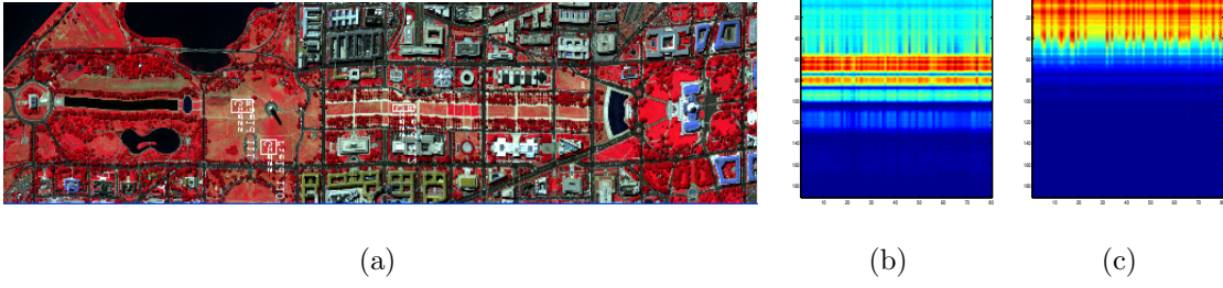
Fig. 5.1. (a) Simulated color IR view of airborne hyperspectral data over Washington DC Mall [64]. (b) Ground-truth pixel spectrum of grass. (c) Ground-truth pixel spectrum of water.
